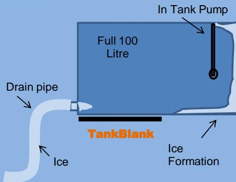
Tests were performed in a cold chamber environment at -15 °C for a period of 16 hours. The exercise demonstrated that Ice will form on the inside of the tank as shown in the diagrams above. But if TankBlanket and the water system elements are positioned and installed correctly the system continues to work.
